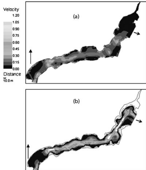
Figure 4. Calculated water velocities before (a) and after (b) complete weir removal at  $15 \text{ m}^3 \text{ s}^{-1}$  discharge on the lower reach. Arrow indicates inflow and outflow directions.
