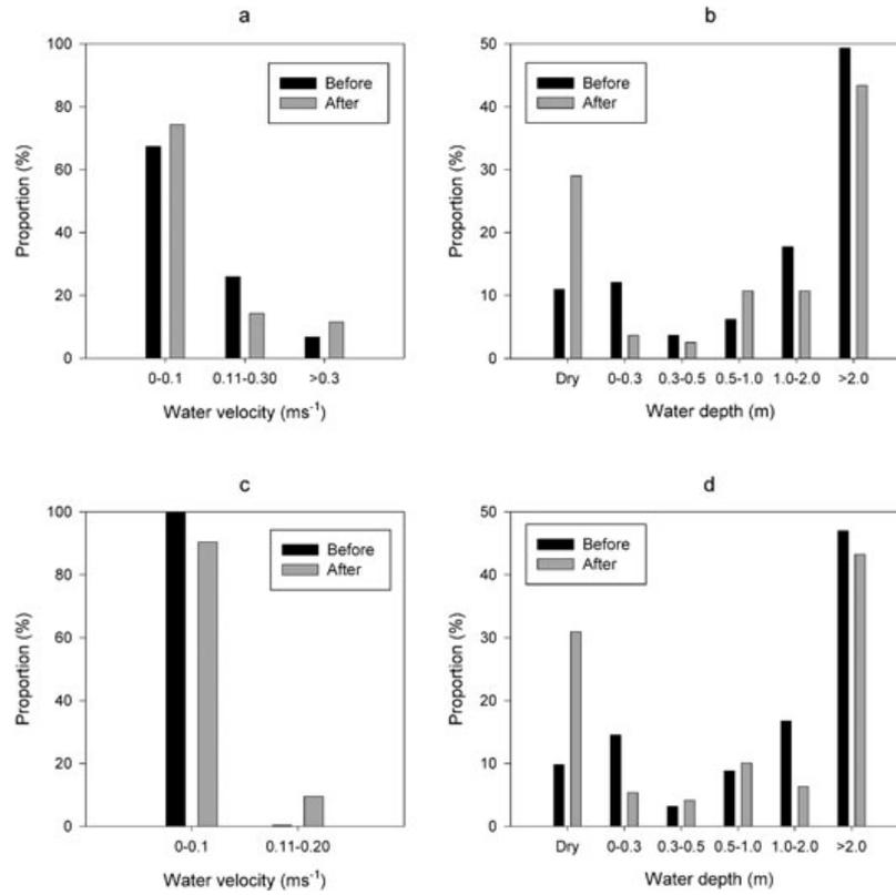
Figure 5. Calculated water velocities and depths before and after weir removal at  $15 \text{ m}^3 \text{ s}^{-1}$  (a and b) and  $3 \text{ m}^3 \text{ s}^{-1}$  (c and d) on the upper reach. Dry cells are omitted in the velocity distribution figures.
