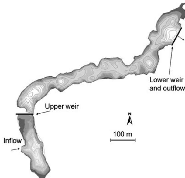
Figure 2. Bathymetric map with bed-level contours (interval = 1 m). The map covers wetted area at a discharge of 15 m<sup>3</sup> s<sup>-1</sup> before removal of the two weirs. The dam at Rygene hydropower station is situated around 400 m upstream from the inflow to the study site.
