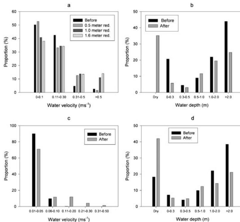
Figure 3. Calculated water velocities and depths before and after weir removal at 15 m<sup>3</sup> s<sup>-1</sup> (a and b) and 3 m<sup>3</sup> s<sup>-1</sup> (c and d) on the lower reach.
